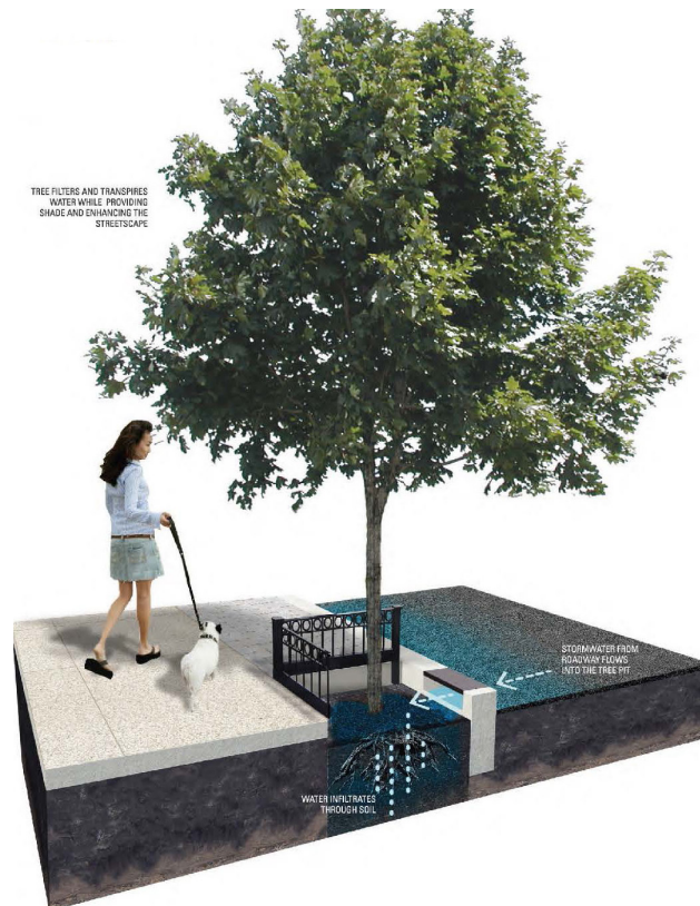
Stormwater tree pit diagram Source: Philadelphia Water Department, water.phila.gov
